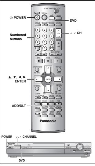
After plugging the unit into your household AC outlet and pressing [ $\bigcirc$  **POWER**] to turn the unit on for the first time, the unit assists you to set the menu language, and automatically tunes in all the channels it can receive and sets the clock.
