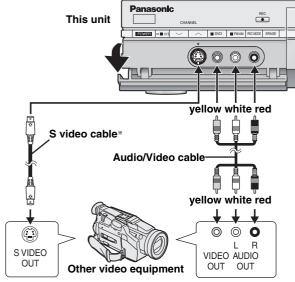
If the audio output of the other equipment is monaural, connect to L/ MONO. (Both left and right channels are recorded when connected through L/MONO.) Connecting to the input terminals on the rear of the unit, L1 or L3
