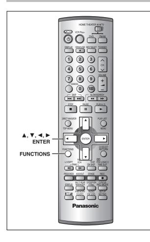
By using the FUNCTIONS window you may access the main functions quickly and easily.
