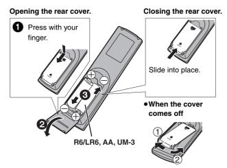
•Insert so the poles (+ and -) match those in the remote control. • Do not use rechargeable type batteries.
